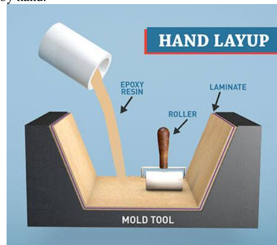
Figure 1. Hand Lay-Up Process
